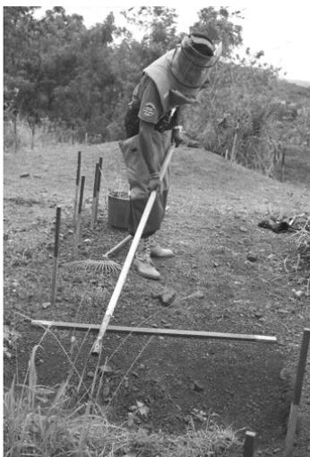
Users have expressed amazement at the ease of use and the low weight of the SD Heavy-rake. The tubular stainless steel handles are lighter than many wooden handles. The picture on the left shows a deminer raking in an area with heavy vegetation and hard, rocky ground.
